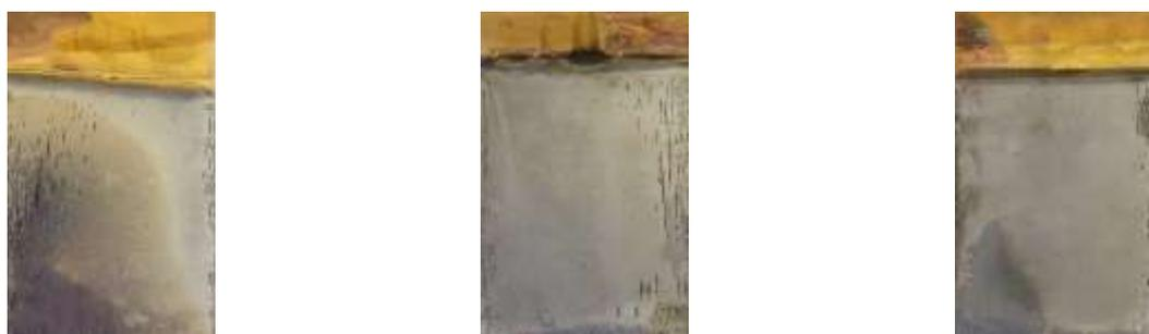
г)  $i = 2,5 \text{ A/dm}^2$ ,  $T = 20 \text{ }^\circ\text{C}$  д)  $i = 3,0 \text{ A/dm}^2$ ,  $T = 20 \text{ }^\circ\text{C}$  в)  $i = 3,5 \text{ A/dm}^2$ ,  $T = 20 \text{ }^\circ\text{C}$
