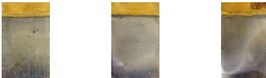
а)  $i = 1,0 \text{ A/dm}^2$ ,  $T = 20 \text{ }^\circ\text{C}$  б)  $i = 1,5 \text{ A/dm}^2$ ,  $T = 20 \text{ }^\circ\text{C}$  в)  $i = 2,0 \text{ A/dm}^2$ ,  $T = 20 \text{ }^\circ\text{C}$
