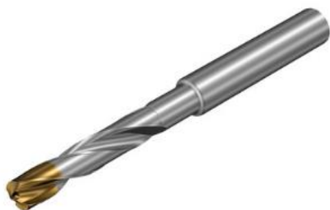
Рисунок 1.7 – Сверло CoroDrill 860.1-0850-044A0-GM X1BM ( M8, D_c = 8,5, LU = 44, SIG = 140, PL = 1.547, OAL = 103, LF = 101,453, LCF = 61 )
