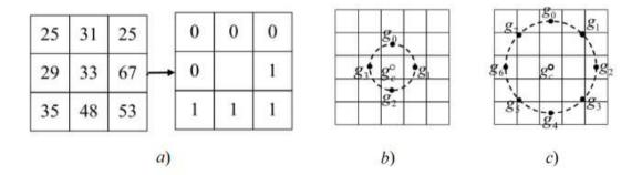
Fig. 3. An example of LBP operator calculation
