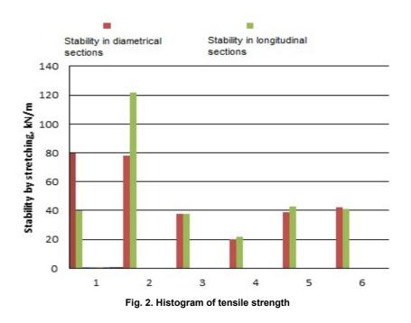
results are exceeded using the displacement of specific density in giving directions. All results are presented in histogram in Fig. 3 [8].
