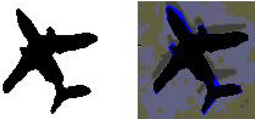
Fig. 3. Measurement of aircraft area for a filter mask n = 5 and conversion threshold \theta = 0,6 (left), and an imposition of the image area (left) to the real aircraft image (right)
